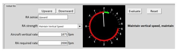
Figure 14: Data entry and RA display for a Maintain Vertical Speed RA.
