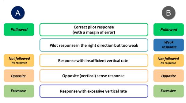
Figure 3: Response classification for "Method A" and "Method B"
