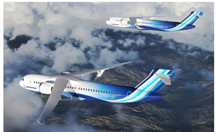
Transonic Truss-Braced Wing concept from the Sustainable Flight Demonstrator project © Boeing
