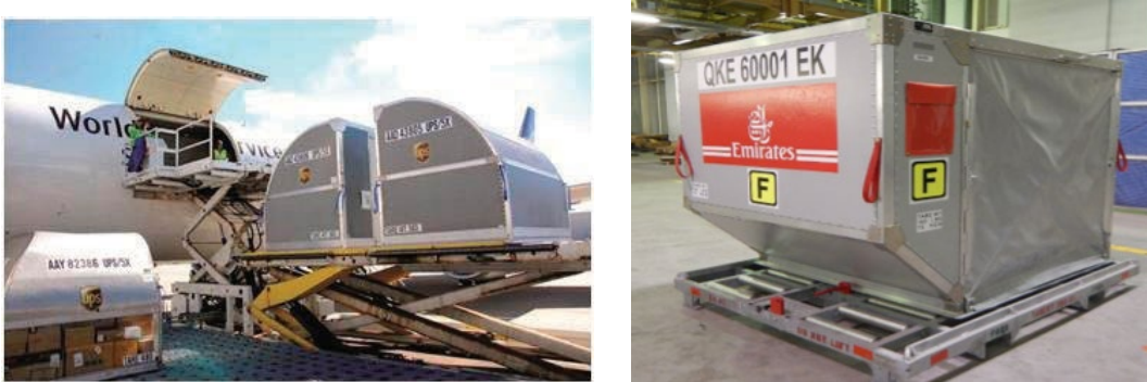
Figure 14 – Main deck and lower deck fire-resistant containers
