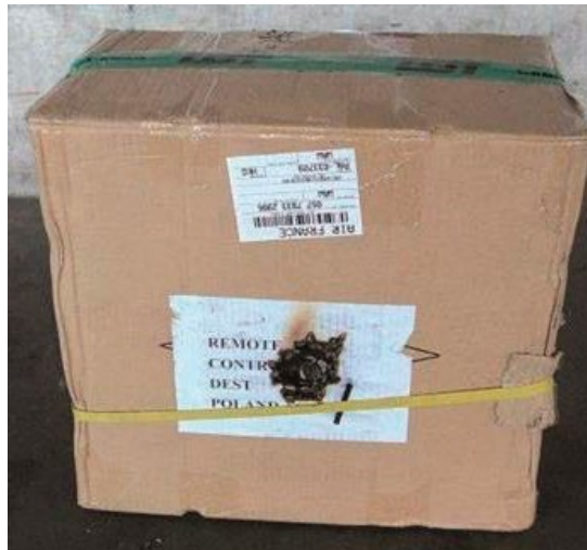
Figure 1 – Fire damage to a package of incorrectly packed lithium metal button cells, which occurred after unloading from an aeroplane
