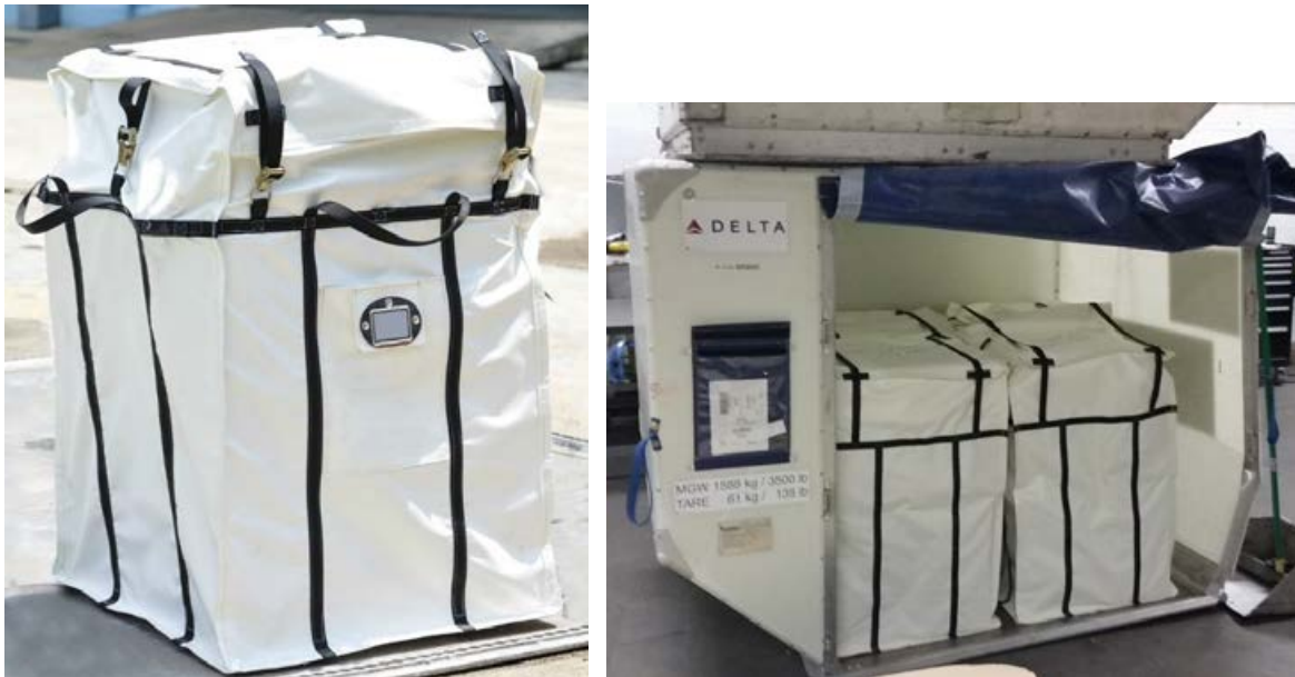
Figure 16 – Fire containment bags loaded on a certified aircraft pallet and in a certified lower deck aircraft container
