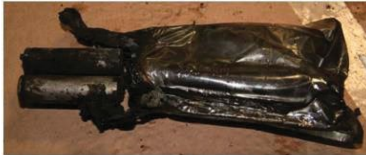
Figure 2 – A non-compliant laptop battery ordered online and sent by airmail, which caught fire shortly after being unloaded from a passenger aircraft
