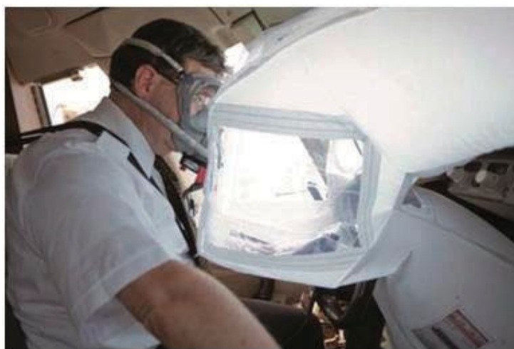
Figure 12 – Smoke displacement system (EVAS – Enhanced vision assurance system)
