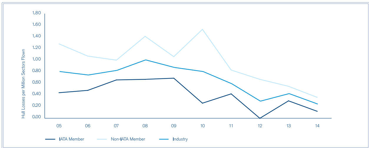
Jet Aircraft Hull Loss Rate: IATA Member Airlines vs. Non-IATA Member Airlines and Industry (2005-2014)
