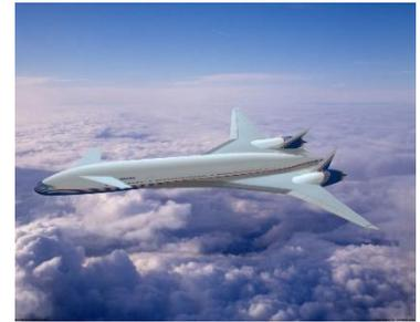
**Blended wing:** Wide airfoil-shaped bodies and efficient high-lift wings enable significant lift-to-drag ratio improvements compared with conventional aircraft. High fuel savings are generated as the entire plane is designed to generate lift.
