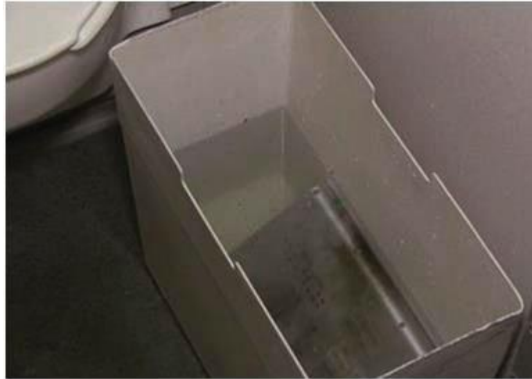
Figure 23 – The toilet waste bin with water holding the damaged device should be stowed and isolated in a toilet
