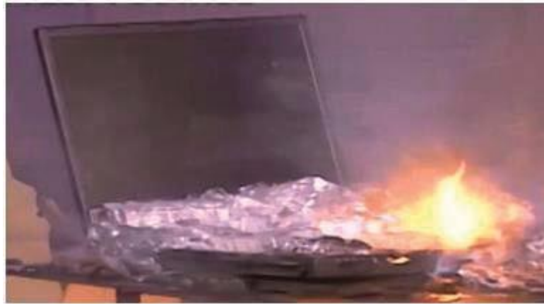
Figure 21 – A demonstration of the effect of applying ice to a burning laptop
