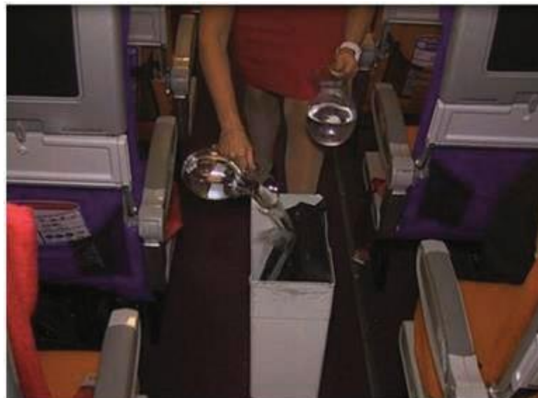
Figure 22 – A laptop in a bag being immersed in water inside a toilet waste bin
