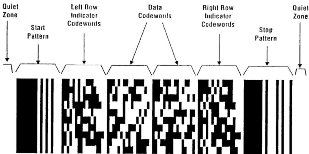
Figure 21 - Structure of the PDF417 symbol as defined in the ISO/IEC 15438
