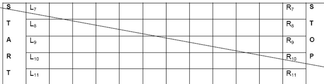
Figure 23 - Schematic showing a scan line crossing rows of the PDF417 symbol
