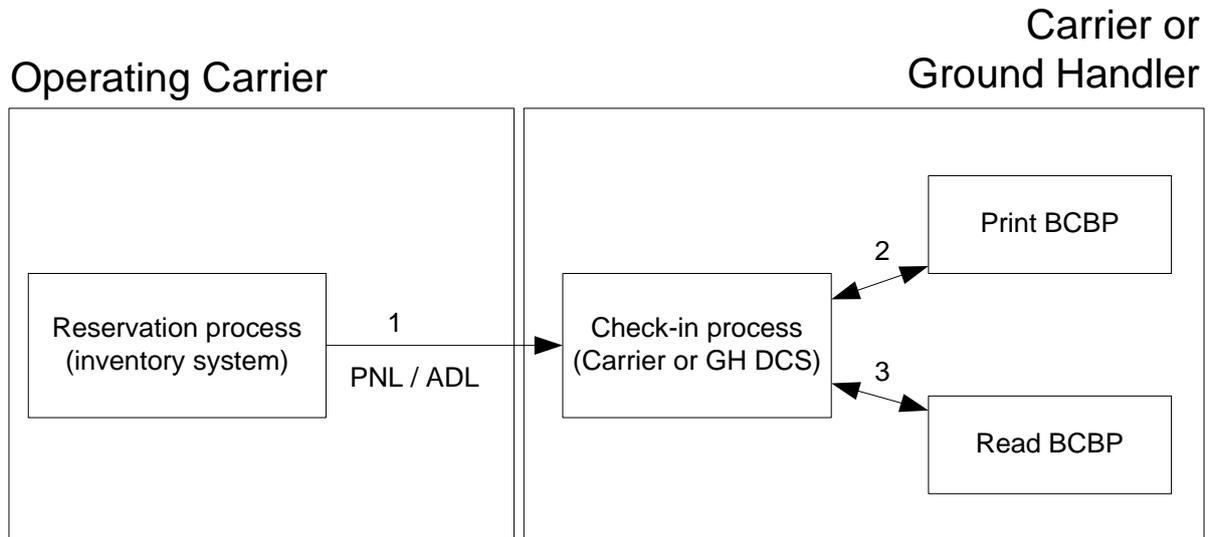
Figure 6 - Data flow of passenger information at check-in
