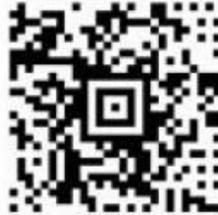
*Figure 4 - Example of an Aztec code courtesy of Air France / KLM*
