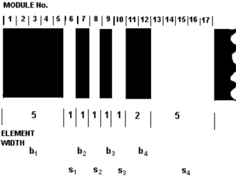
Figure 22 - PDF417 is composed of 4 elements whose widths add up to 17 modules
