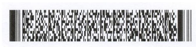
*Figure 3 - Example of a PDF417 bar code courtesy of British Airways*
