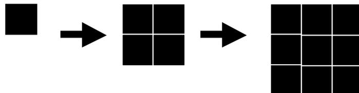
Figure 7 - One bar code cell displayed in 1, 2 or 3 pixel width
