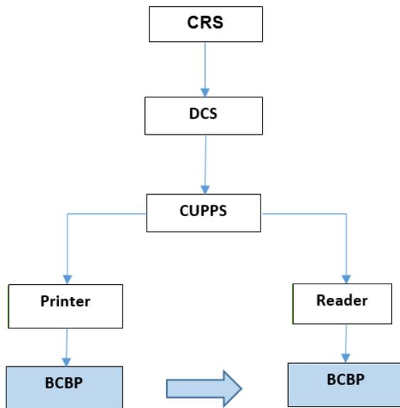
*Figure 9 - Data flow in a CUPPS environment*
