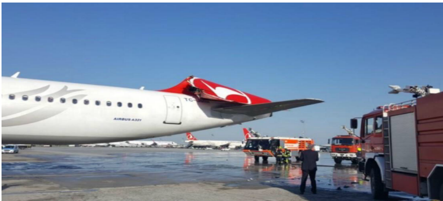
Turkish Airlines A321 had its horizontal stabilizer impacted by with another aircraft
