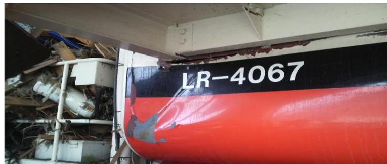
Figure 43-Photo showing broken tank of the fueller at receiving bay to park.
