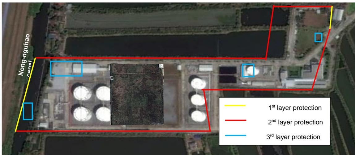
**Level 1:** Improvement for existing flooding protection system e.g. 50 cm added dike, access road protection, reservoir and pumping station.
