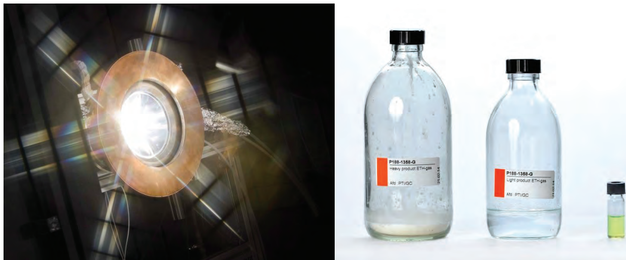
Figure 10 – Solar-thermochemical reactor at ETH Zurich (left picture) that was used for the first-ever production of “solar kerosene” in the EU-FP7 project SOLAR-JET. Products of the StL (Sun-to-Liquid) process are shown in the right picture (from left to right flask): Heavy FT products (waxes), liquid FT products and middle distillate (jet fuel range) products of hydrocracked sample of FT waxes. The bright green color of the latter (“solar kerosene”) probably originates from trace amounts of metal catalysts from the hydrocracking procedure. (Source: http://www.solar-jet.aero ).
