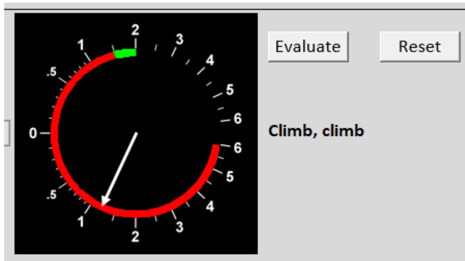
Figure 13: Representation of RA display on the IVSI.
