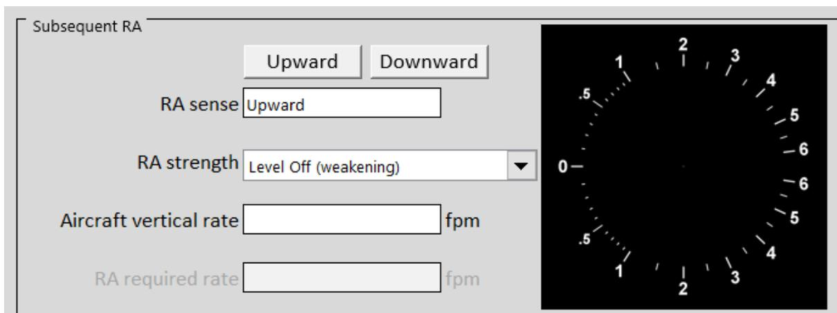
Figure 12: Subsequent RA details entry space.
