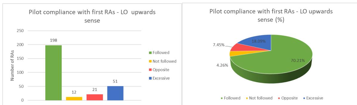
Figure 17. Pilot Compliance with first Level Off upwards RAs – 16 seconds duration.
