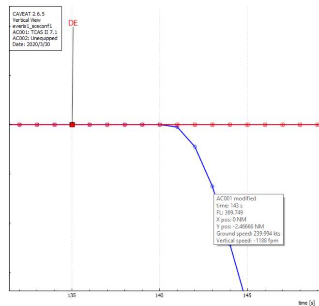
Figure 1: Simulation results 8 seconds after an RA was generated.
