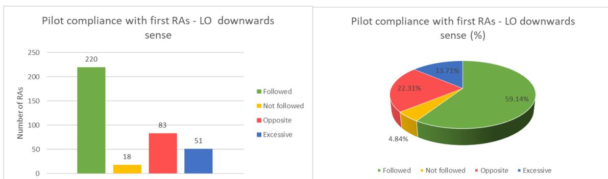
Figure 12. Pilot Compliance with first Level Off downwards sense RAs – 12 seconds or longer.
