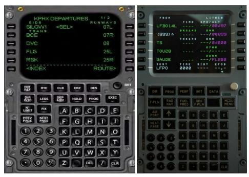
Figure 2: Typical FMS Control & Display Units (CDU)
