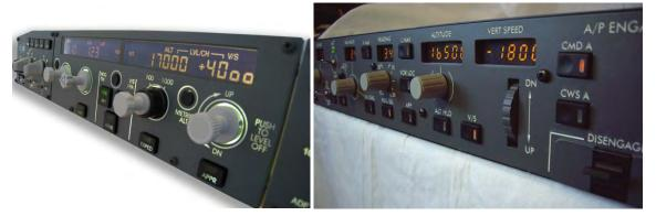
Figure 3: Typical Glareshield Autopilot/Flight Director Interfaces
