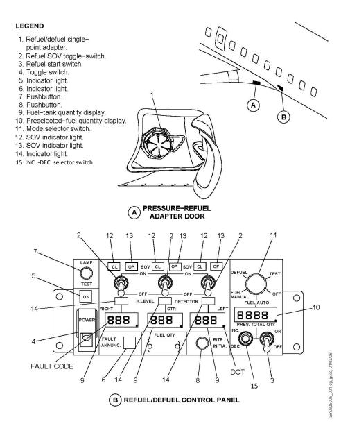
Note: Label for item 15 (INC-DEC selector switch) has been added to diagram B.
