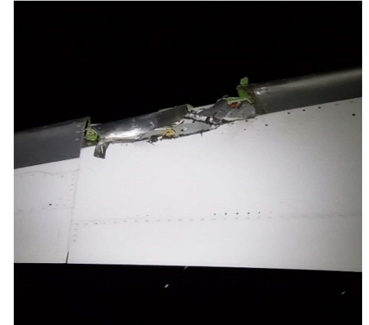
B787-900 raked wingtip The only repair option, with proprietary bonding techniques USD 1,500,000
