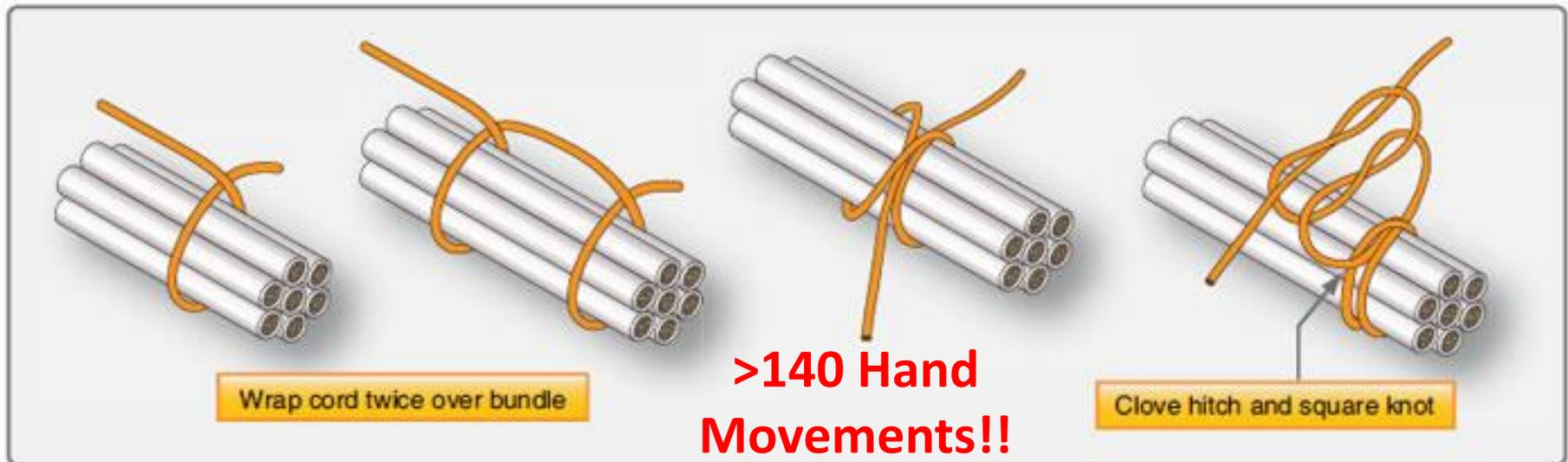
**LaceLok<sup>®</sup>** – A new option for secondary support of cable bundling
