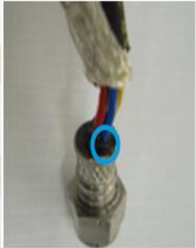
(3) Examples of Harness and Outb Skew Sensor with sealant applied
