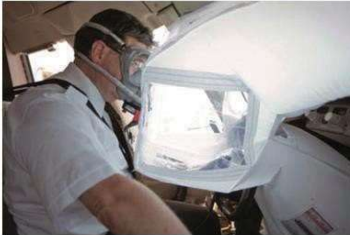
Figure 14 – Smoke displacement system (EVAS – Enhanced vision assurance system)
