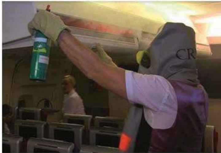
Figure 19 – Discharging a fire extinguisher into an overhead locker
