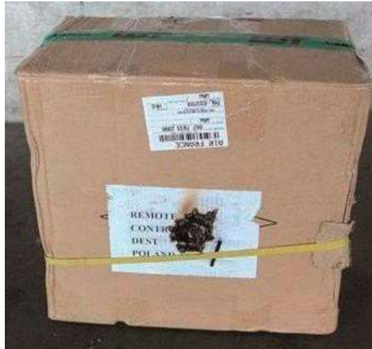
Figure 5 – Fire damage to a package of incorrectly packed lithium metal button cells, which occurred after unloading
