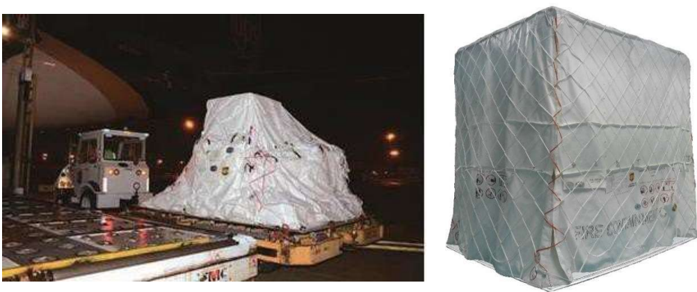
Figure 12 – Fire containment cover for lower deck and main deck deployment
