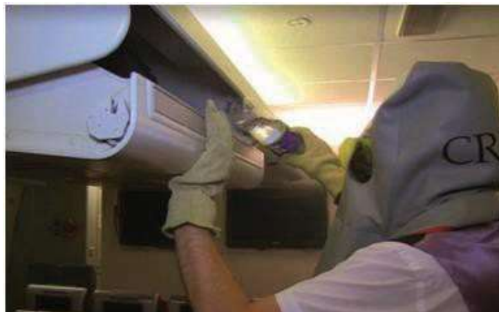
Figure 21 – Applying water to a burning device without removing it from the overhead locker. It is important to note that liquid may turn to steam when it is applied to heated batteries.
