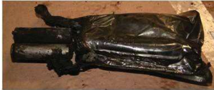
Figure 6 – A non-compliant laptop battery ordered online and sent by airmail, which caught fire shortly after being unloaded from a passenger aircraft at London Heathrow Airport
