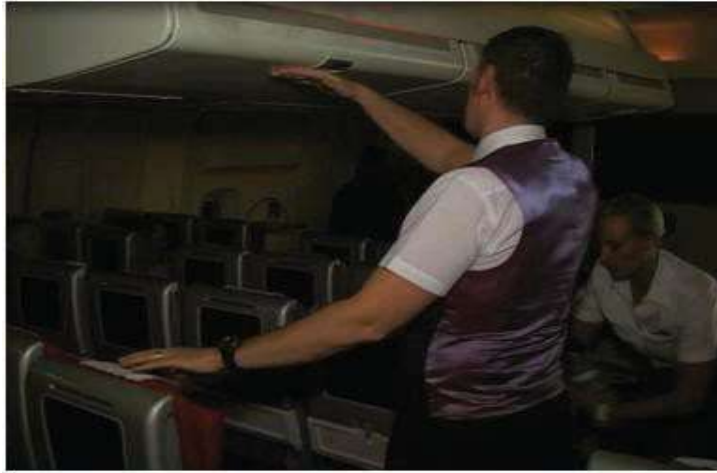
Figure 18 – Determining the location of a fire in an overhead locker. After first considering the use of PPE, a fire extinguisher should be discharged into the locker.
