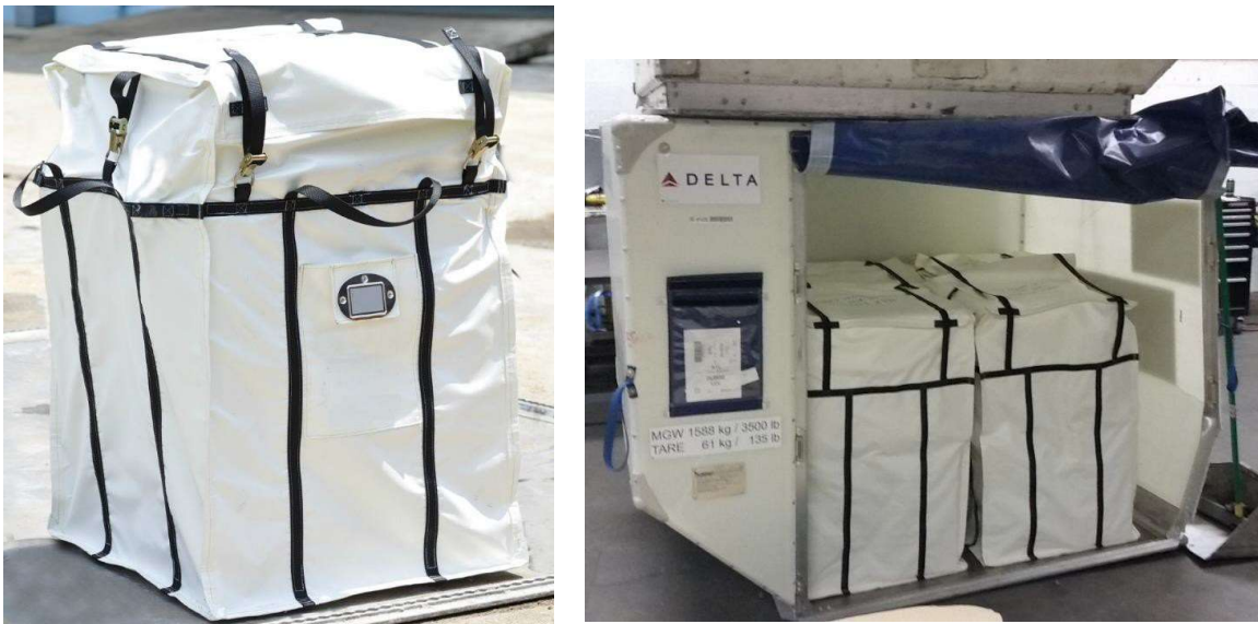
Figure 13 – Fire containment bags loaded on a certified aircraft pallet and in a certified lower deck aircraft container
