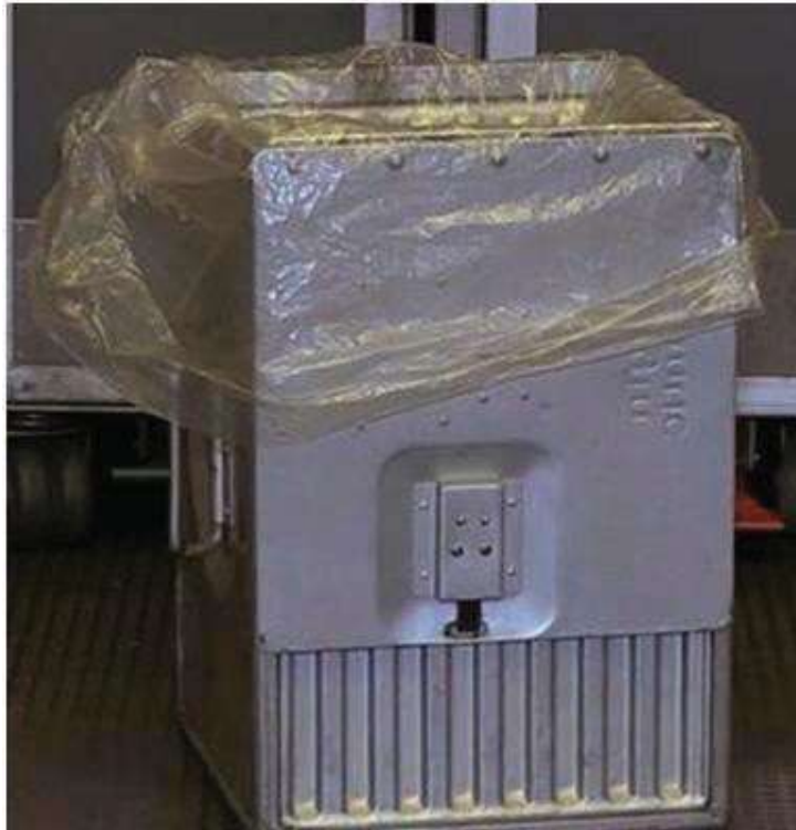
Figure 25 – A bar box made watertight by using a plastic bin liner
