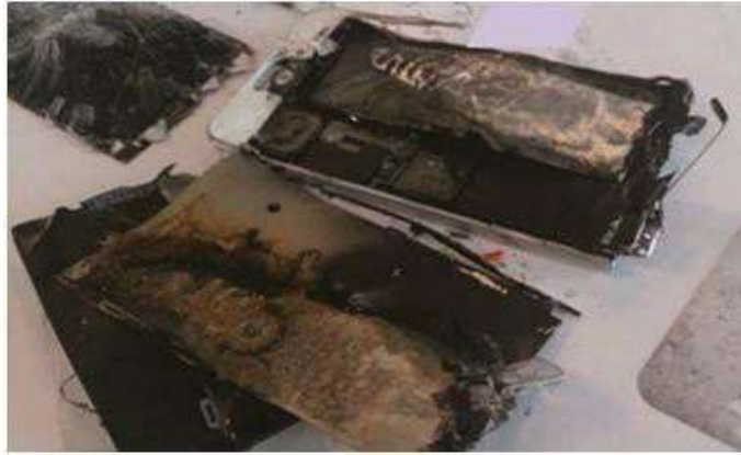
Figure 27 – The charred remains of a mobile phone
