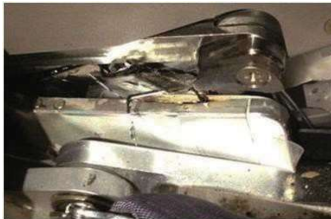
Figure 26 – A mobile phone crushed in an electrically adjustable seat
