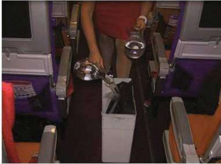
Figure 23 – A laptop in a bag being immersed in water inside a toilet waste bin
