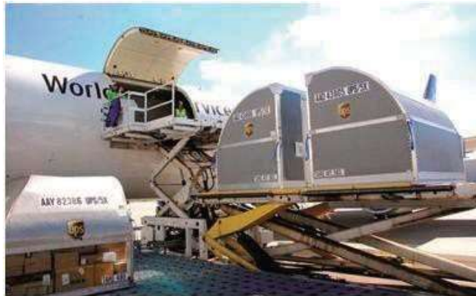
Figure 11 – Main deck fire-resistant containers
