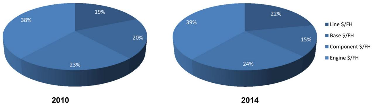
**Figure 1.** Direct Maintenance Cost Structure by Segment; Evolution 2010-2014
