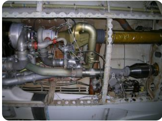
Condenser & heat exchanger
