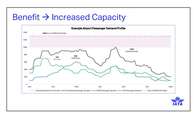
One of the key drivers behind these efficiencies is the fact that, in most airports, international and domestic passenger peaks typically occur at different times. Designing infrastructure to accommodate each peak separately often leads to significantly larger requirements than if we sized for a **combined peak**.
