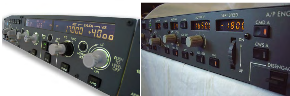
Figure 3: Typical Glareshield Autopilot/Flight Director Interfaces
