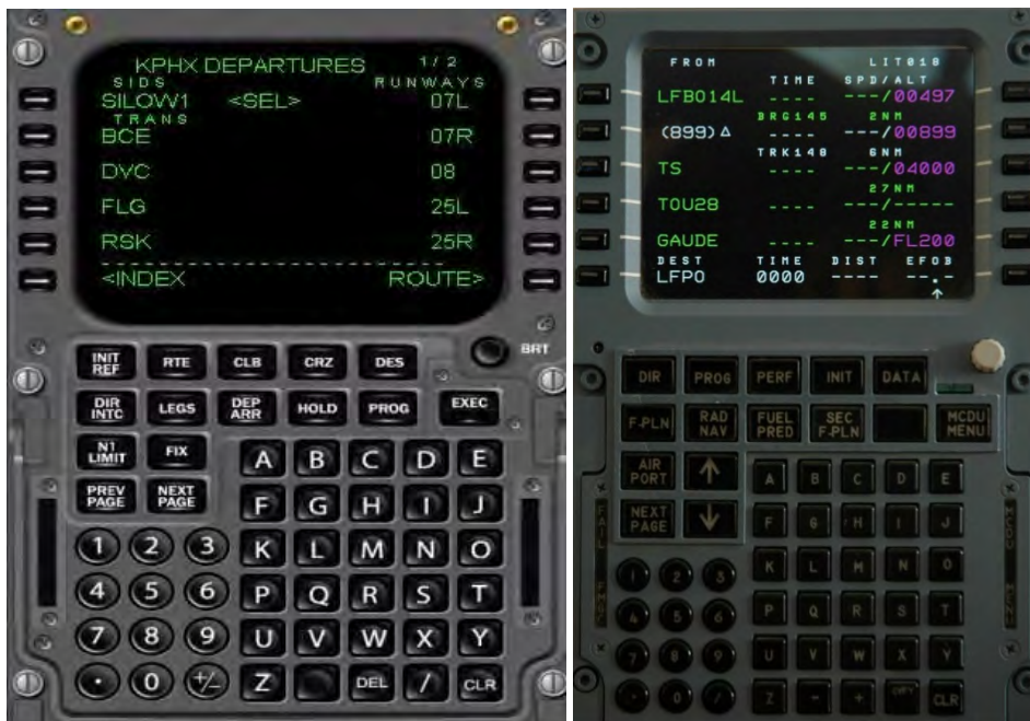
Figure 2: Typical FMS Control & Display Units (CDU)
