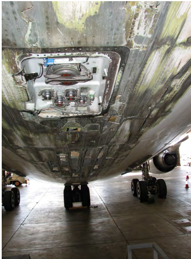
Figure 1: A340 Tailstrike Damage
